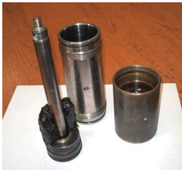
FIGURE 3-18. High-Viscosity Heavy Oil Acquired by Wireline Sampling
